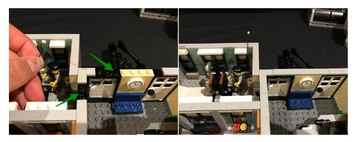
119. Take the entire top level and then then turn it on its side to allow us to be able to install another 2 LED strip lights (striplight#6 and striplight#7) to the following positions. Connect a 15cm cable in between the 2 strip lights and then connect a 30 cm cable to the other port on striplight#7.
