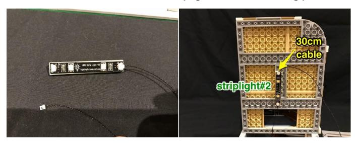
78. Connect the connecting cable from the level below into the other port on striplight#2 and thread the 30cm cable connected to the other port up the open space which leads to the 3rd level.
