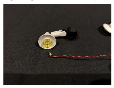
31.Place the LED component facing upward inside the middle of the trans yellow piece of one of the lamps. Pull the cable over the top of the lamp and then pull it right toward the black brick. Reconnect this lamp section back to the front wall ensuring the cable is tight and in between the 2 black bricks.
