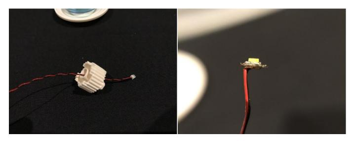
14.Pull the cable all the way through from the other side so that the LED component is right up against the inside of the white round piece then reconnect the dark grey brick with yellow technic pin through the top of the white round piece. Your base of the fountain section with blue dot light installed should look similar to the below example.
