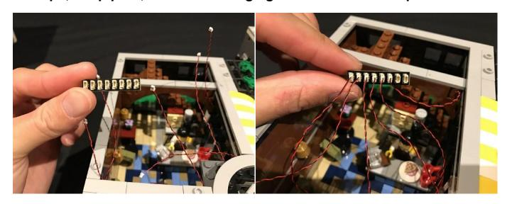
50. This is a good time to test our current light circuit. To do so, insert 3x AA batteries to the battery pack and then connect the battery pack cable into a spare port of the expansion board. Turn on the battery pack and verify that all the lights connected to the cafe are currently lit.
