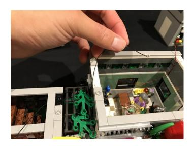
54. Secure and hide the cable underneath the grey tiles on the top of each building floor.
