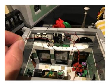
107. We will now test the lights we have installed so far as well as adjust the speed of the flicker effect for the fountain. Take the battery pack and connect the battery pack cable into any of the spare ports of one of the expansion boards. Turn on to verify all is working ok.
