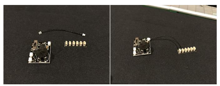
101. This multi effects board has 3 different effects. For this light kit, we will be using effect# 3 (flicker effect). Set it to the 3rd option by flicking the switch to the far right. We will later use the wheel on the effect board to adjust the speed of the flicker effect as desired.
