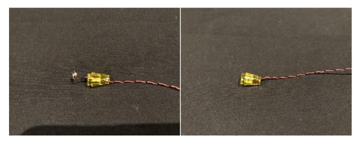
91.Reconnect the trans yellow piece with dot light installed back to the lamp section ensuring the cable is facing toward the back.
