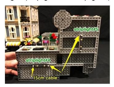
110.Connect a 15cm connecting cable in between the 2 strip lights, another 15cm connecting cable to the left port of striplight#4 and a 30cm connecting cable to the bottom port of striplight#5.
