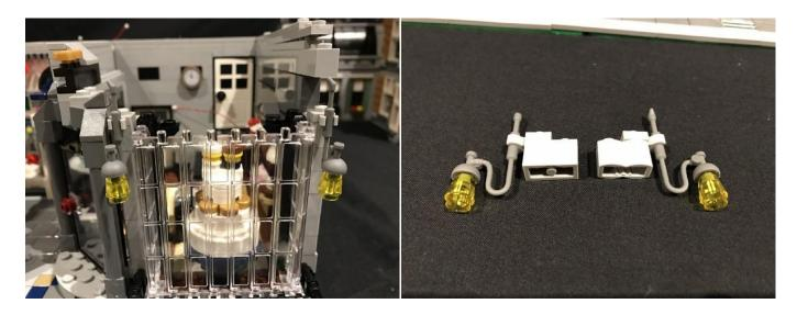
88.Disconnect the trans yellow piece from each of the lamp sections. Take a Dot Light with 15cm cable and thread the connector side through the larger hole of the trans yellow piece. Thread it all the way through but before the LED component reaches the piece, bend the component part 90 degrees upward so that the LED component is facing up toward the inside, then pull the cable all the way through.
