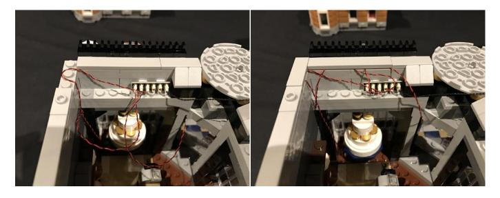
100. Take the Multi Effects Board and then connect this to another 6-port Expansion board using a 5cm connecting cable. Connect the cable into the port on side of the effects board which only has one port.
