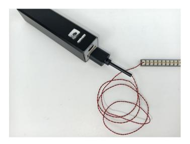
When we test "A02508 Light Strip-Red" particles, Take out the bag labelled "A02508 Light Strip-Red". Take out one of the light and connect it to the socket. Turn on the power bank, the light will turn on normally as shown below.
