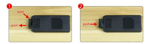
All our connections between plug and socket are all the same as shown above. So for any such structure with plug and socket, please pay attention to the golden wire of the plug and the golden needle of the socket, they must be touched together.
