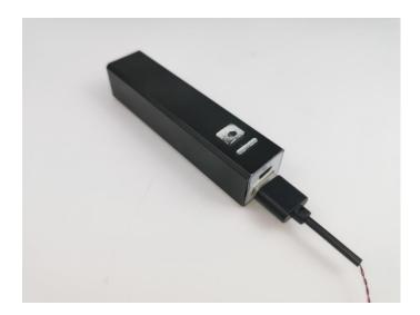
When we test "Flash Light-30CM Red" particles, Take out the bag labelled "Flash Light-30CM Red". Take out one of the light and connect it to the socket. Turn on the power bank, the light will turn on normally as shown below.
