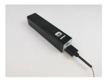
When we test "Light-15CM Warm White" particles, Take out the bag labelled "Light-15CM Warm White". Take out three of the light and connect it to the socket. Turn on the power bank, the light will turn on normally as shown below.
