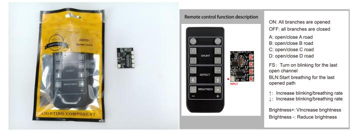
The remote control does not contain batteries, please buy a 2025 or 2032 button battery in the nearest store and install it in the remote control.
