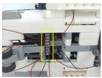
Twist the longer lighting wire into a single strand and put it in the slot.
