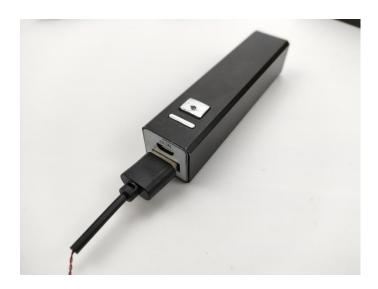
When we test "Light-30CM Red" particles, Take out the bag labelled "Light-30CM Red". Take out one of the light and connect it to the socket. Turn on the power bank, the light will turn on normally as shown below.
