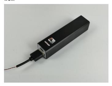
when we test "30cm 2x3 Double row light bar-Warm White" particles, Take out the bag labelled "30cm 2x3 Double row light bar-Warm White". Take out one of the light and connect it to the socket. Turn on the power bank, the light will turn on normally as shown below.
