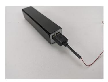
when we test "High-Brightness Light 30CM-White" particles, Take out the bag labelled "High-Brightness Light 30CM-White". Take out one of the light and connect it to the socket. Turn on the power bank, the light will turn on normally as shown below.
