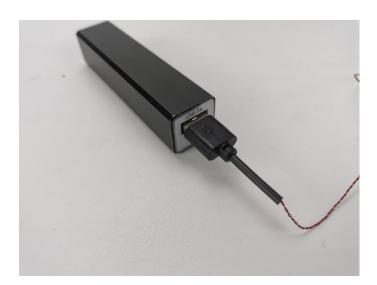
when we test "High-Brightness Light 30CM-White" particles, Take out the bag labelled "High-Brightness Light 30CM-White". Take out one of the light and connect it to the socket. Turn on the power bank, the light will turn on normally as shown below.
