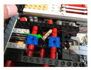
99.Neatly place the expansion board in between sections as per below.
