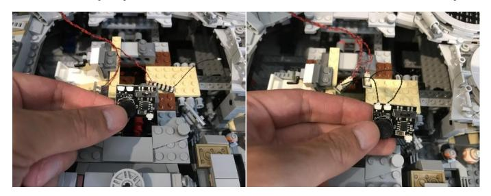
149.We now need to setup the chosen effect on the Multi Effects Board. First turn on the Battery Pack and then set the switch on the multi effects board to the middle (we will be using the emergency effect to display as the shooting canon effect). Turn the effect dial all the way to the left for the slowest effect. You should now see the upper cannons firing away in sequence.
