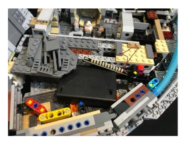
18.We will now light the interior cabin section closest to the back. Start by disconnecting the corridor section to the left.
