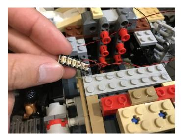
75.Take another White 30cm Dot Light and this time connect the connector side first into the next available port on the 6-port expansion board. Leave the Dot Light end as is for now as we will stick this end to the roof of the middle section later.
