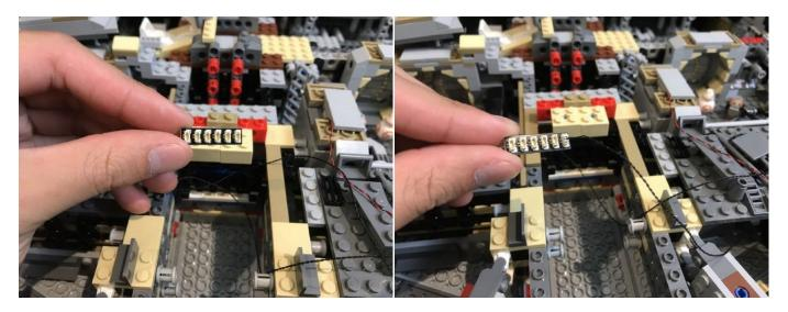
53.Take the Multi-Effects Board and connect the other 30cm connecting cable we pulled across to the input port on the board (side with only one port).
