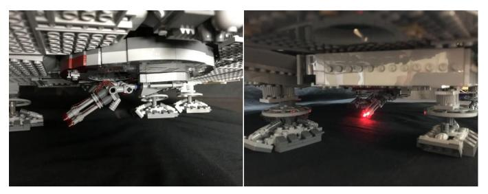
162.Before reconnecting the main round roof section above, neatly tuck the expansion boards, effects board, and any excess cabling into the middle section.
