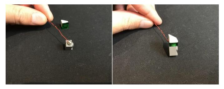
29.Thread the connector side of the flashing dot light behind in the space between the technic bricks before reconnecting this control panel section.
