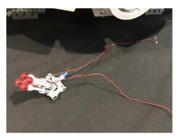
140.Take 2x 6-Port Expansion Boards and 2x 5cm Connecting Cables. Connect a 5cm cable to each expansion board and then connect 2 dot lights from each cannon to each expansion board as shown below.
