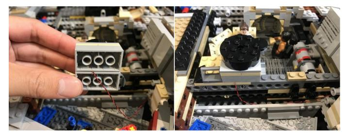
72.Pull the cable behind and toward the right. Thread it thought the space which leads to the other side and then thread it underneath, up toward the middle before reconnecting it to the 6-port expansion board.
