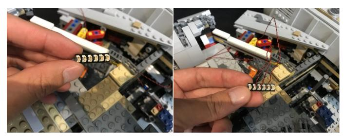
116.Locate the other end of the 30cm connecting cable from the expansion board earlier (step 35) and connect this to an available port.
