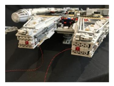
92.Pull the cable from the front left side across to the right toward the inside and secure it underneath the dark grey bar as shown below before connecting the Dot Light into the 6-port expansion board.
