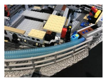
15.Take the AA Battery Pack and insert 3x AA batteries to it. Connect the battery pack cable to the 12-port expansion board and then turn the battery pack ON to test the lights for the back jets.
