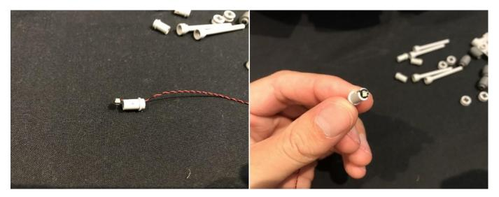
126.Take one of the provided Trans Red 1x1 Round Plate and connect it directly over the top of the Dot Light to secure it in place.
