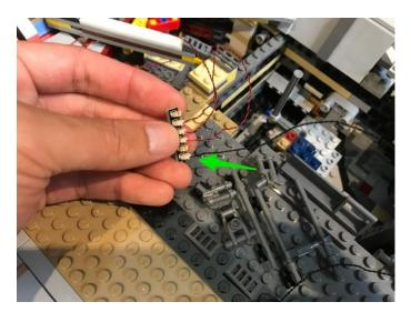
117.Neatly place the expansion board inside the middle compartment and then turn the Battery Pack on to test all lights are working so far.
