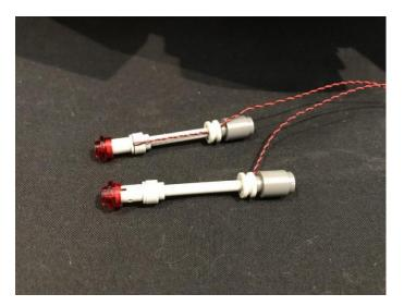
131.Reconnect the 2 cannons with lights to the cannon base. Connect one on the top left and the other on the bottom right ensuring the cables are facing the same way as per below.
