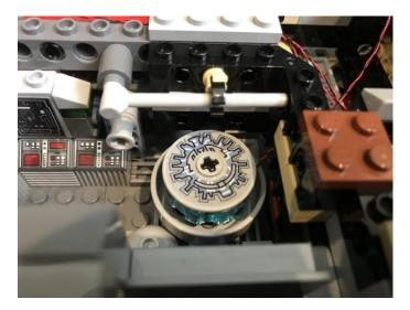
38.Thread the cable from the hyperdrive dot light through the black Technic hole (to the right of the hole we threaded the 2 dot light cables earlier). Pull the cable all the way through and then connect it to the 12 port expansion board.
