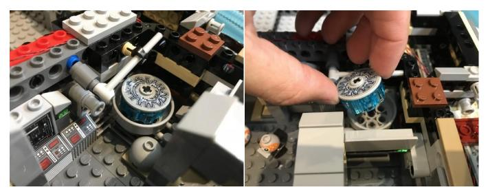
35.Take a White 30cm Dot Light and thread the connector side through the hole of the black technic brick in the corner. Pull the cable all the way through from the other side and then stick the Dot Light down (LED facing up) in the following position using an adhesive square.
