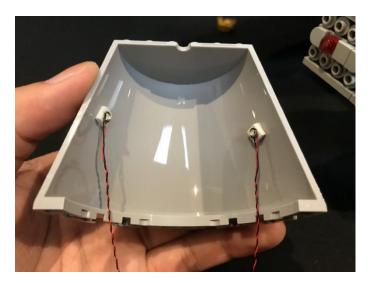
109.Reconnect the section underneath the cockpit and thread all cables underneath and then along the right side.
