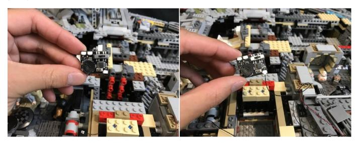
54.Place the multi-effects board down the middle section as shown below.
