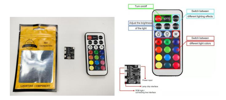
The RGB remote control does not contain batteries, please buy a 2025 or 2032 button battery in the nearest store and install it in the RGB remote control.
