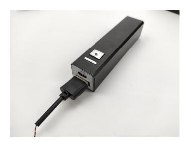
when we test "Light Strip-Warm White" particles, Take out the bag labelled "Light Strip-Warm White". Take out one of the light and connect it to the socket. Turn on the power bank, the light will turn on normally as shown below.
