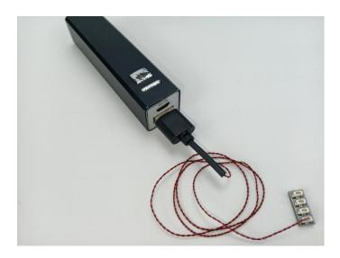
when we test "High-Brightness light 30CM-Warm White" particles, Take out the bag labelled "High-Brightness light 30CM-Warm White". Take out one of the light and connect it to the socket. Turn on the power bank, the light will turn on normally as shown below.
