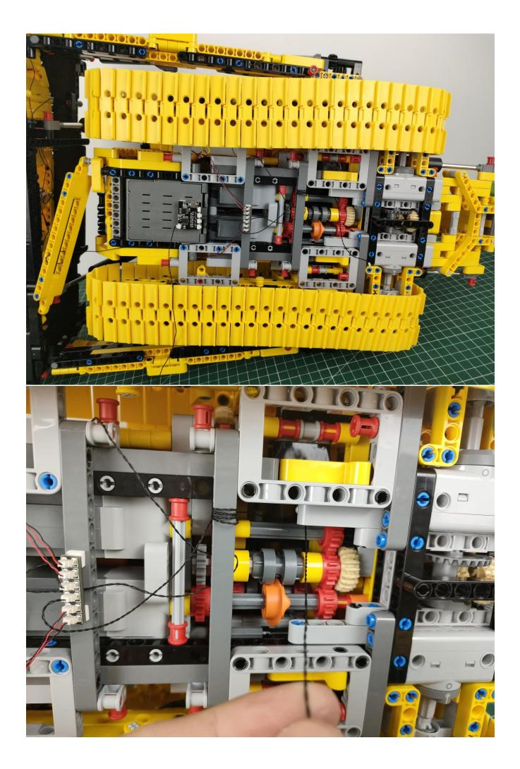
Put the connecting wire through the small hole of the gray building block first, then pull the connecting wire to the left, continue to wrap the longer connecting wire around the gray building block, and finally connect the connecting wire to the remote control module.
