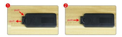
The connection method between the USB Power Cord and RGB Remote Control Module is as follows:
