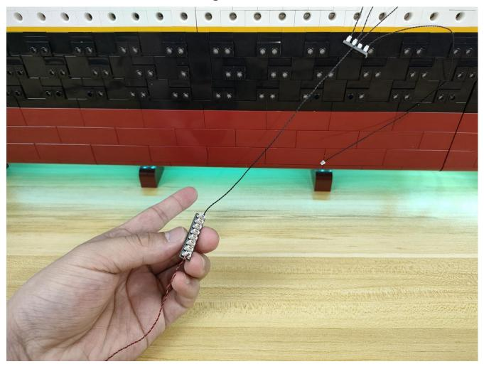
Then remove the connecting wire of the atmosphere light at the bottom of the hull and connect it to the four expansion board.
