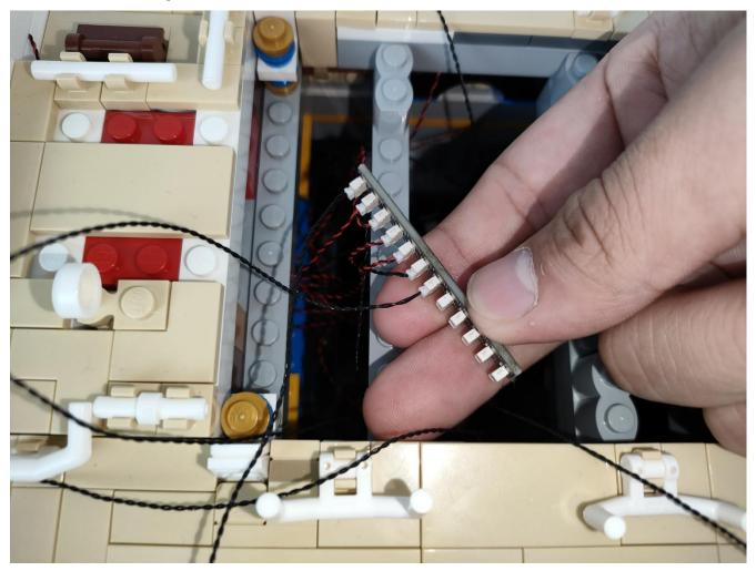
Then unplug the 20cm cable on the 12 expansion board from the power supply.
