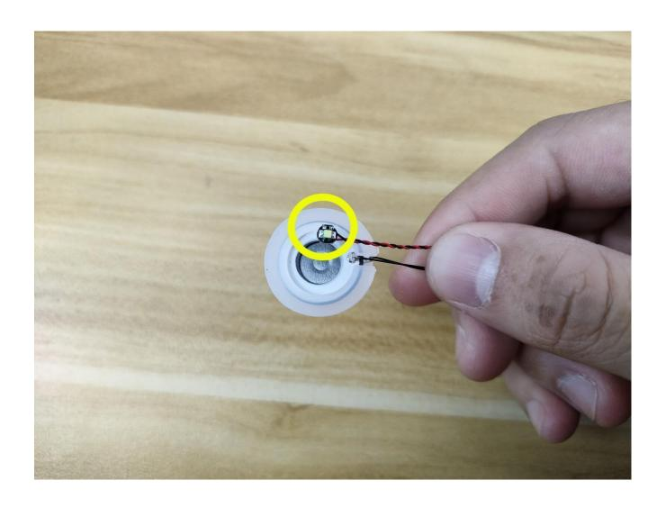
Fix the lamp pellet at the position selected by the frame in the figure, with the solder joints of the spray module components facing upwards.
