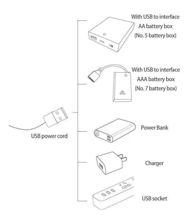
Connect the USB power cord to the mobile power supply (the power supply is self-provided, this article uses the mobile power supply, other power supply methods are shown in the figure above).
