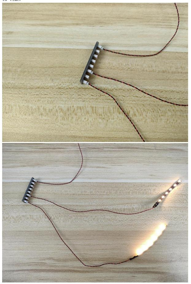
Pull out the lighting after the test is normal. After there is no abnormality, first temporarily put the lighting back into the original bag, and prepare to test other lighting parts. In order to prevent the lighting from not bright after installation, the lighting in other bags are also tested in the same way. After testing a bag, please temporarily put it back in the original bag to avoid confusion with each other.
