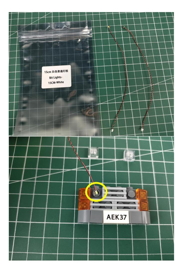
Fix the transparent building blocks on the lamp pellets. The light grain line is at the oblique angle of the square building block.
