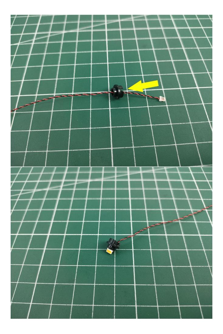
The lamp thread is stuck in the cut of the small circular plate.
