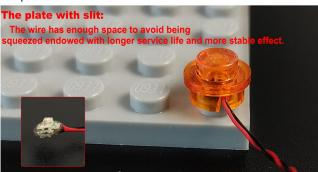
The slit on the the plate round 1X1 are hand-made to avoid squeeze the wire and cause short circuit and abnormalheat during installation.
