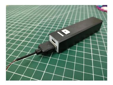
when we test "Light Strips-Blue-7" particles, Take out the bag labelled "Light Strips-Blue-7". Take out two of the light and connect it to the socket. Turn on the power bank, the light will turn on normally as shown below.
