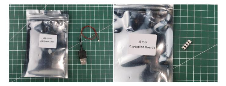
It is worth reminding that our products are all customized. They have a unique way of connecting. The white plug on wire and the socket of the expansion board need to be connected together to transmit power.
