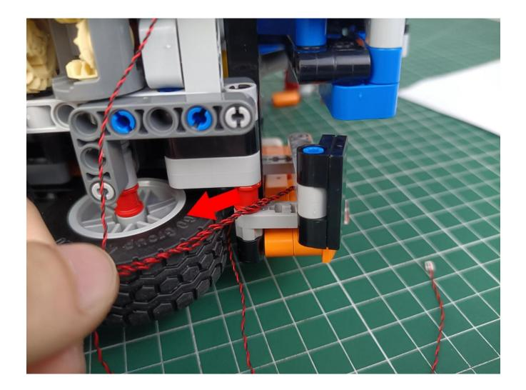
Please pay attention to the way the interface is used. The interface is small, please use it carefully: the = sign of the 2P interface is aligned with the = sign of the expansion board
