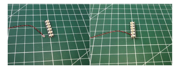
when we test "Bit Lights-15CM-White" particles, Take out the bag labelled "Bit Lights-15CM-White". Take out one of the light and connect it to the socket. Turn on the battery box, the light will turn on normally as shown below.
