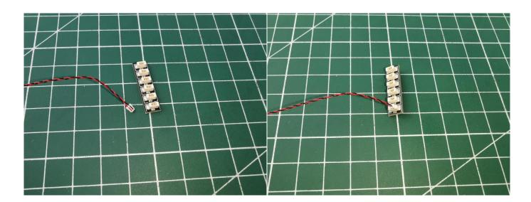
when we test "Multi-Colour Light String" particles, Take out the bag labelled "Multi-Colour Light String". Take out two of the light and connect it to the socket. Turn on the switch on the battery box, all the lights are on as shown.
