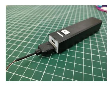
when we test "Bit Lights-15CM-Red" particles, Take out the bag labelled "Bit Lights-15CM-Red". Take out one of the light and connect it to the socket. Turn on the power bank, the light will turn on normally as shown below.
