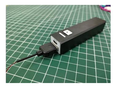
when we test "Bit Lights-15CM-Warm White" particles, Take out the bag labelled "Bit Lights-15CM-Warm White". Take out one of the light and connect it to the socket. Turn on the power bank, the light will turn on normally as shown below.
