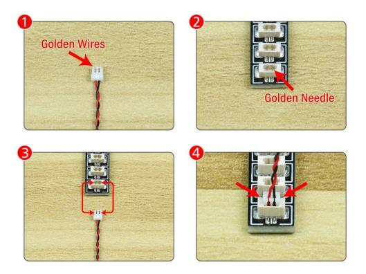
All our connections between plug and socket are all the same as shown above. So for any such structure with plug and socket, please pay attention to the golden wire of the plug and the golden needle of the socket, they must be touched together.
