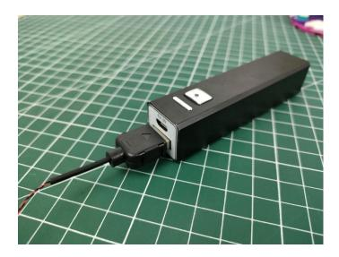
when we test "Bit Lights-30CM-Red" particles, Take out the bag labelled "Bit Lights-30CM-Red". Take out one of the light and connect it to the socket. Turn on the power bank, the light will turn on normally as shown below.
