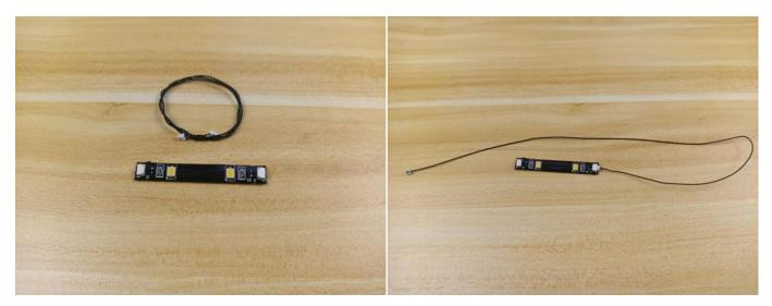
87.Connect the connecting cable to the other end of the strip light.
