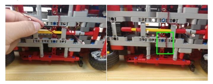
.Take a 30cm connecting cable, an 8-port expansion board, assemble the as per below.
