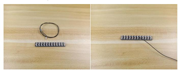
.Connect the following taillights cables to the expansion board.
