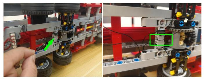
.And connect it to the D port on the Remote Control Switch Board.c
