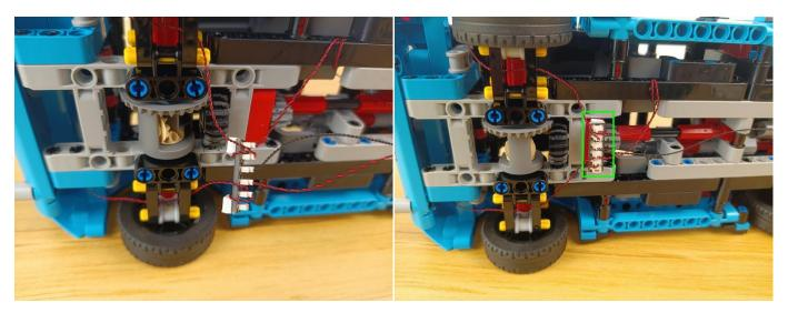
**51.**Tighten excess cables up as per below.
