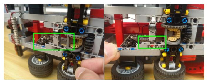
.Connect the connecting cable to the A port.
