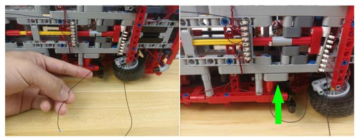
**149**.Wind it around the following piece before connecting it to the expansion board.
