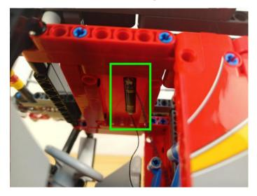
**90**.Turn to the side, thread the cable through the following hole and tighten it up.
