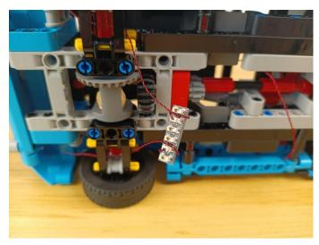
**44.**Thread the cable from the roof inside through the following space.
