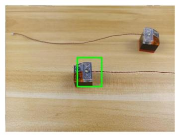
**68.**Thread the cable to the bottom, reconnect the headlight to the right.
