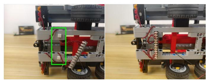
.Thread the connecting cable from the expansion board through the following hole and wind around the following piece.
