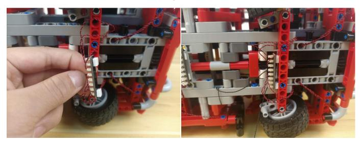
**152**.Pull the connecting cable from the expansion board to the left.
