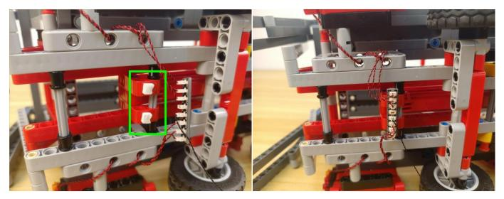
. Thread the connecting cable through the following 2 holes.
