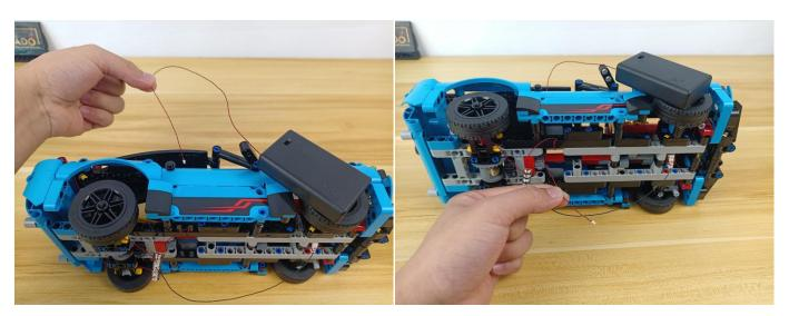
**48.**Connect the cable from the battery pack to the 6-port expansion board.
