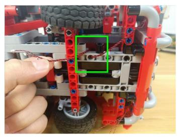
145.Group the cables underneath together as well, and wind them around the piece.
