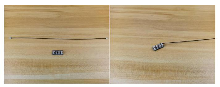
**34.**Connect the following 2 cables to the expansion board, you can tuck excess cables around the expansion board.
