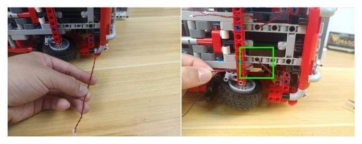
**146**.Take a 30cm connecting cable, an 8-port expansion board, assemble the as per below.
