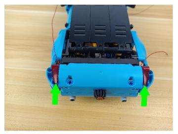
**27.**Thread the cable through the following space, and pull it out from the bottom.
