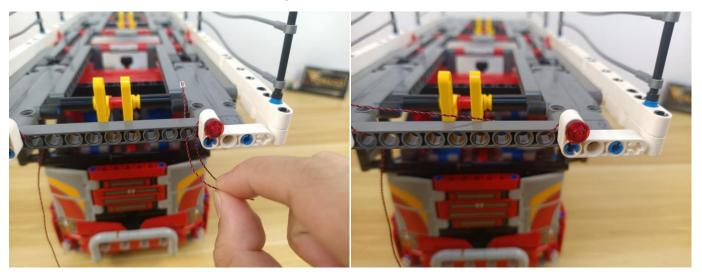
.Pull the cable to the left, and thread it through the following hole.
