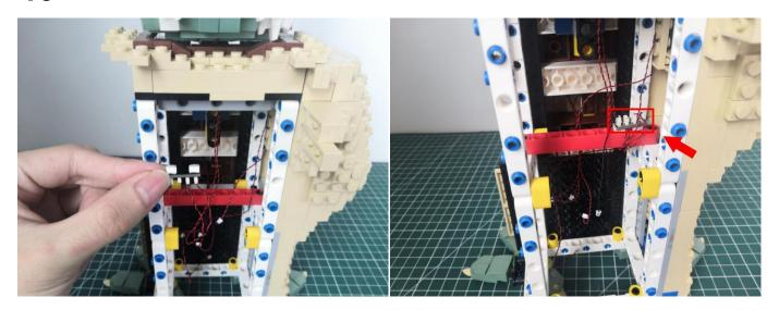
Take a 6-port expansion board, a 5cm connecting cable, connect the connecting cable the expansion board.
