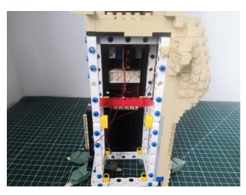
Take a 5cm connecting cable, a 4-port expansion board, connect the connecting cable the expansion board.
