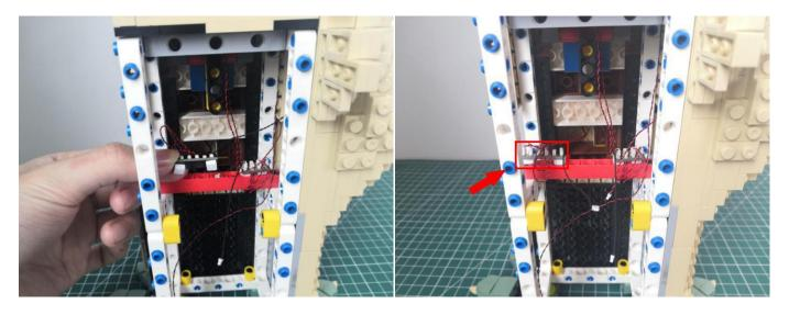
Take an AAA battery pack, a Remote Control Switch Board, connect the cable of the battery pack to the Remote Control Switch Board as per below.
