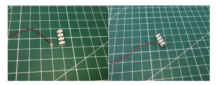
when we test "Bit Lights-30CM-Red" particles, Take out the bag labelled "Bit Lights-30CM-Red". Take out two of the light and connect it to the socket. Turn on the power bank, the light will turn on normally as shown below.
