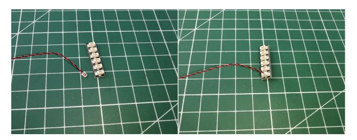
when we test "Bit Lights-15CM-White" particles, Take out the bag labelled "Bit Lights-15CM-White". Take out one of the light and connect it to the socket. Turn on the power bank, the light will turn on normally as shown below.
