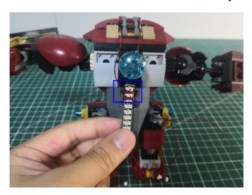
53. Connect the other cables to the expansion board, you can tuck excess cables around the expansion board.
