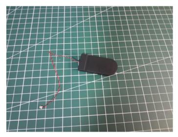
The flat battery pack does not contain batteries, please buy a 2025 or 2032 button battery in the nearest store and install it in the flat battery pack.
