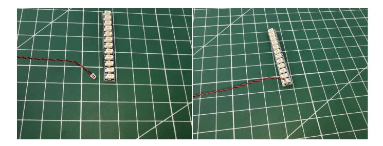
when we test "Bit Lights-15CM-White" particles, Take out the bag labelled "Bit Lights-15CM-White". Take out one of the light and connect it to the socket. Turn on the flat battery pack, the light will turn on normally as shown below.
