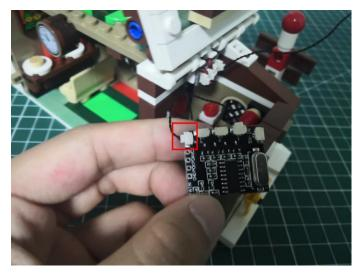
**160.**Connect the following cable from the expansion board to the 3 port.
