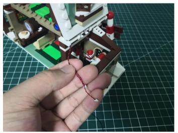
**153.**Connect them to the expansion board, tuck excess cables around the expansion board.
