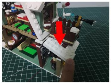
**169.**Connect the connecting cable to the expansion board as per below.
