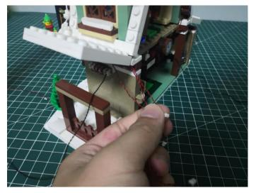
**142.**Connect all the cables to the expansion board, tuck excess cables around the expansion board.
