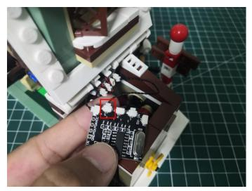
**161.**Connect the cable from the light indoor to the 2 port.
