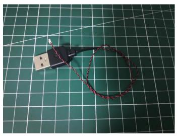
**163.**Connect the USB cable to the input port of the Acousto-optic Control Switch Board.
