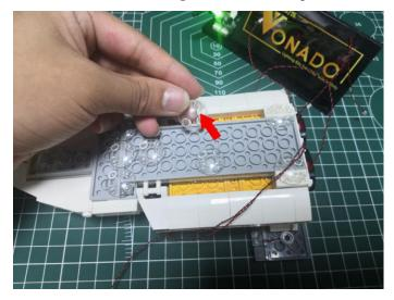
Secure the cables from the spoiler as per below, reconnect the trans round piece,
