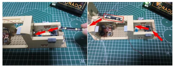
Place the cable underneath the following piece.
