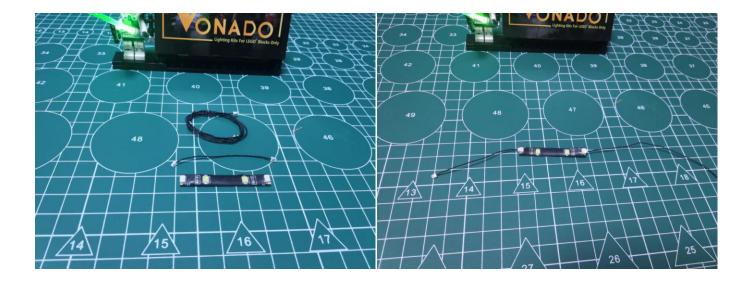
Thread the 5cm connecting cable through the wall, place the strip light as per below.
