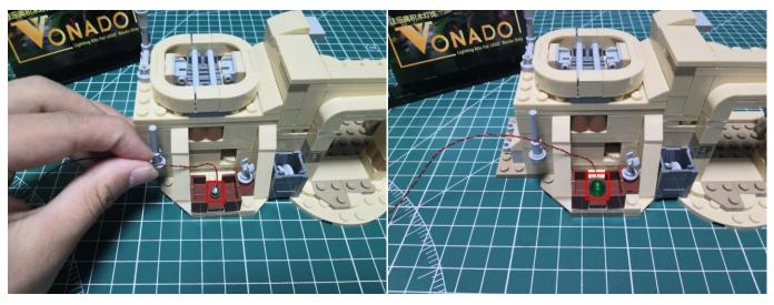
Thread the cable through the following place, pull it out as per below.
