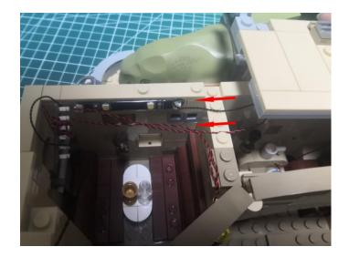
Reconnect the piece, press the 2 cables underneath.
