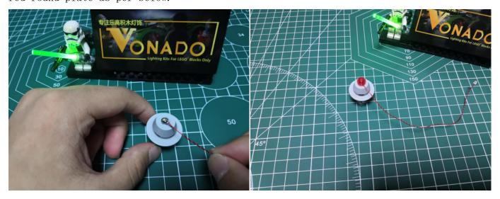
Disconnect the black slope plate and the white piece as per below.
