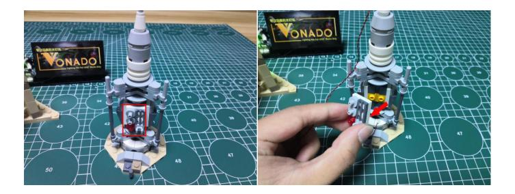
Pull the cable down and straighten the cable.
