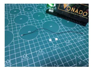
Connect the cable to the expansion board, stick the adhesive squares to the back of the expansion board.
