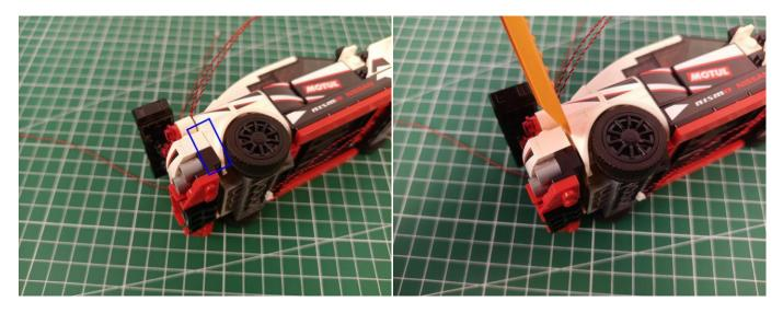
Thread the cables through the gap to the bottom, and close the gap.
