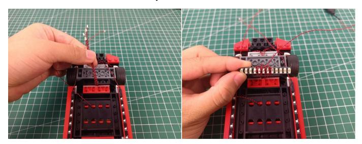
Connect the cables from the strip lights to the expansion board, and tuck excess cables around the expansion board.
