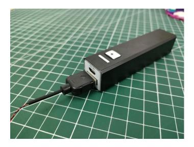
when we test "Bit Lights-15CM-Warm White" particles, Take out the bag labelled "Bit Lights-15CM-Warm White". Take out one of the light and connect it to the socket. Turn on the power bank, the light will turn on normally as shown below.
