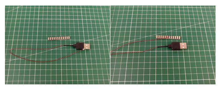
Connect the cables from the tail to the expansion board, and tuck excess cables around the expansion board.
