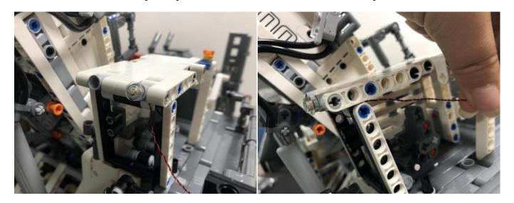
23. Remove the seat, thread the cable through the space underneath.
