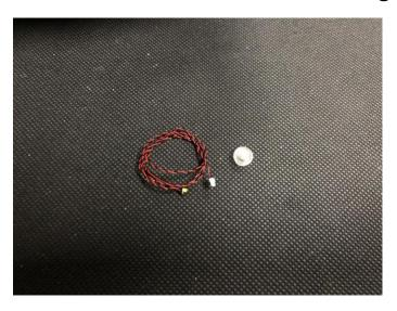
76. Thread the cable through the pin, pull the cable out till the light is placed inside, secure the light with trans piece.
