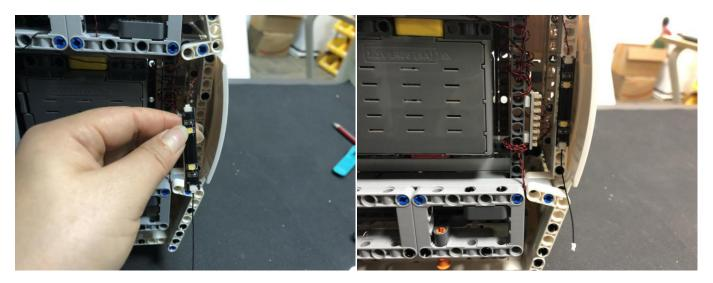
89. Connect the connecting cable from the strip light to the expansion board asper below.
