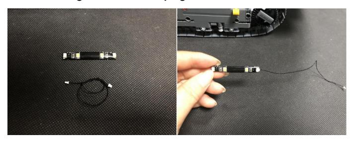
28.Stick the strip light to the roof of the control cabin. Pull the cable backward.
