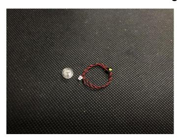
83. Thread the cable through the pin, pull the cable out till the light is placed inside, secure the light with the trans round plate.
