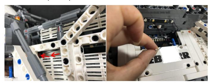
60. Connect the connecting cable to the expansion board.
