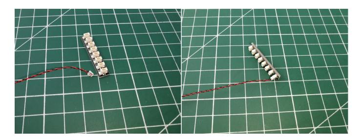
when we test "Bit Lights-15CM-Red" particles, Take out the bag labelled "Bit Lights-15CM-Red". Take out one of the light and connect it to the socket. Turn on the power bank, the light will turn on normally as shown below.
