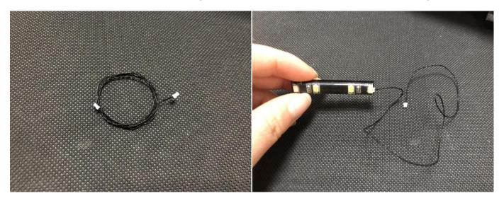
22.Stick the strip light to the roof, reconnect the roof, pull the cable aside, secure it with the roof as per below.
