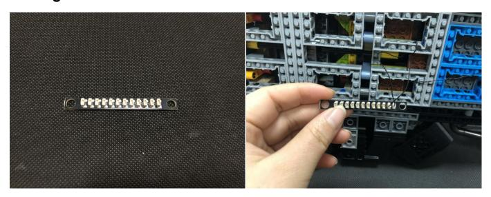
27.Tuck excess cables, connect expansion board to the following place with adhesive squares.
