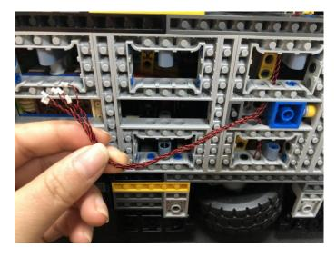
14. Take an 8-port expansion board, connect the 6 cables of the lights to it.
