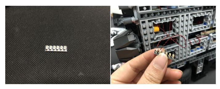
47.Tuck excess cables, stick the expansion board to the following place with adhesive squares.
