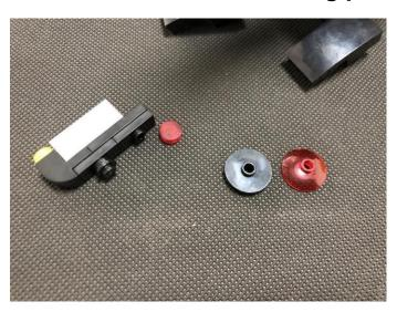
30. Take a 30cm red dot light, thread the light through the black round plate with hoe, pull the cable out till the light is placed against the hole.
