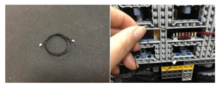
17. Thread the cable through the following holes (thread it as you wish), pull it to the tail of the car.
