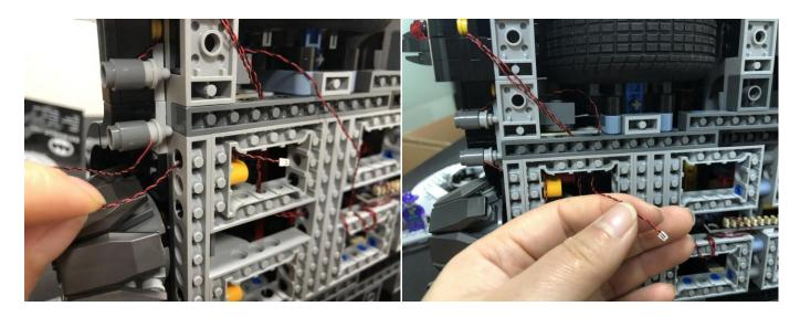
46. Take a 6-port expansion board, connect the 2 cables of the lights to it.
