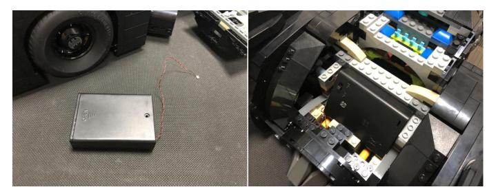
55.Reconnect the piece we removed before, turn the car to its side, pull the cable out from the bottom.
