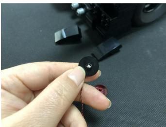
31. Secure the light with the trans red plate.
