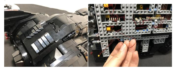
56. Thread the cable of the battery pack through the hole, and connect it to the 12-port expansion board.
