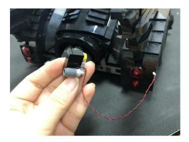
42. Thread the cable through the following space to the bottom of the car.
