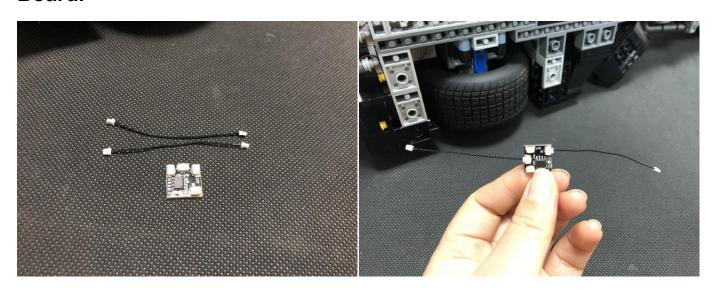
50.Connect the other end of the cable from the output port to the 6-port expansion board, connect the one from the input port to the 12-port expansion board.
