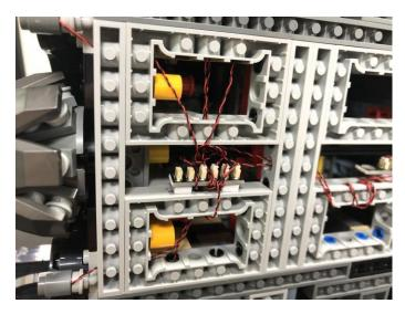
49.Take two 5cm connecting cable, a Flicker Effects Board, connect the two cables to the input and output ports of the Flicker Effects Board.
