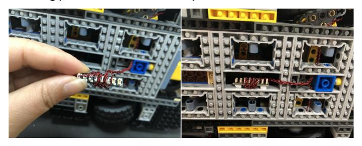
16. Take a 30cm connecting cable, connect it to the expansion board.
