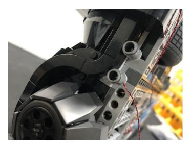
45. Thread the cable through the following place, and pull it out underneath the car.
