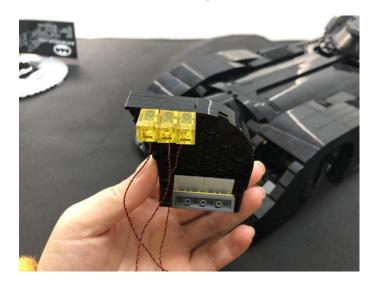
8.Remove the following piece, place the cable between the gray piece.
