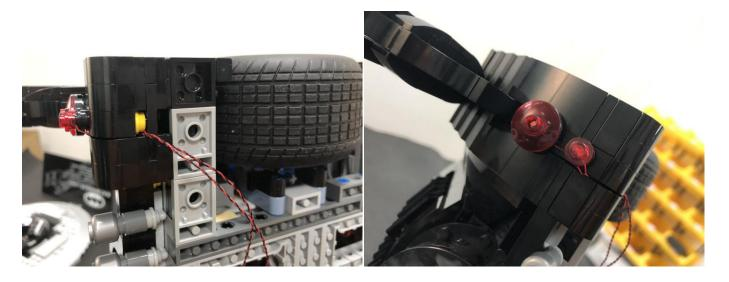
36. Thread the cable through the holes underneath the car(thread it randomly), and pull it to the 12-port expansion board.
