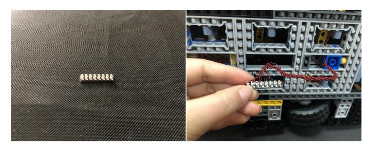
15.Tuck excess cables, and stick the expansion board to the following place with the adhesive squares.
