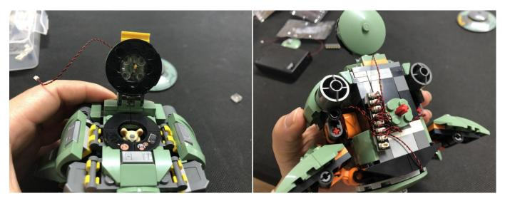
Take the USB cable, connect it to the expansion board.
