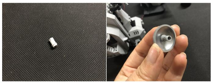
**36**.Take a 30cm flashing blue dot light, thread it connector through the hole, then, pull the cable out
