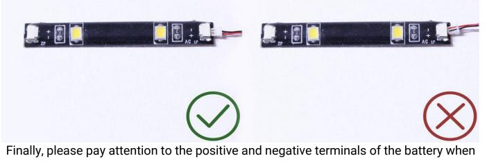
installing the battery case.
