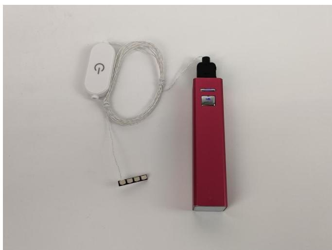
When we test the "①" lighting fixtures, remove one of them and connect it to the socket. Turn on the portable power bank, and the light strip will light up normally, as shown in the figure below.
