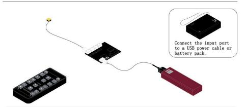
Remove the light fixture from any bag and connect it to the output port of the remote control template.
