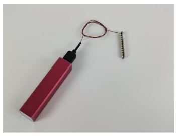
When we test the "⑤" lighting fixtures, remove one of them and connect it to the socket. Turn on the portable power bank, and the light strip will light up normally, as shown in the figure below.
