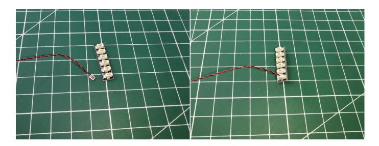
when we test "Bit Lights-30CM-White" particles, Take out the bag labelled "Bit Lights-30CM-White". Take out one of the light and connect it to the socket. Turn on the power bank, the light will turn on normally as shown below.
