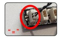
Connect the AAA Battery Pack to the 6-Port Expansion Boards.
