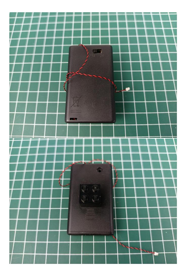
Open the power cover of the AAA Battery Pack and install the battery.(Pay attention to the positive
