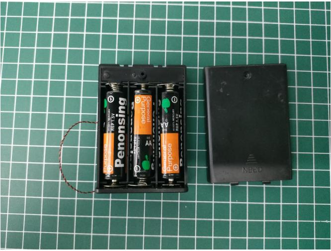
Install 3 AA batteries (note the positive and negative poles).
