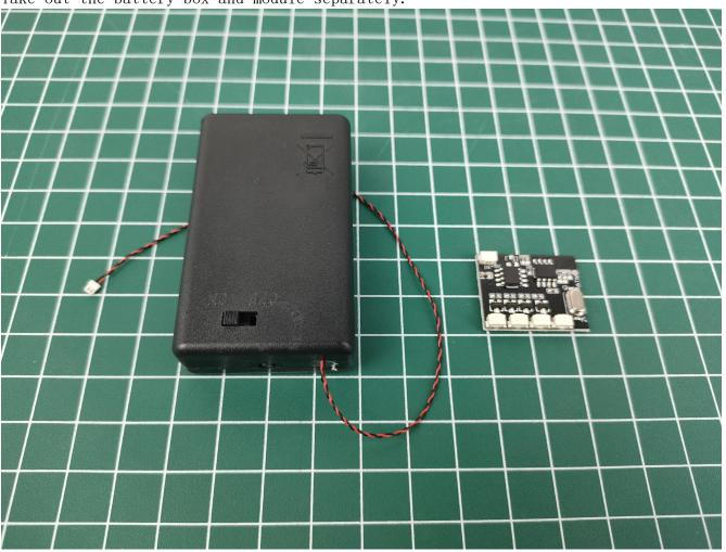
Connect the 2P terminal wire of the battery box to the module, paying attention to the position and method.
