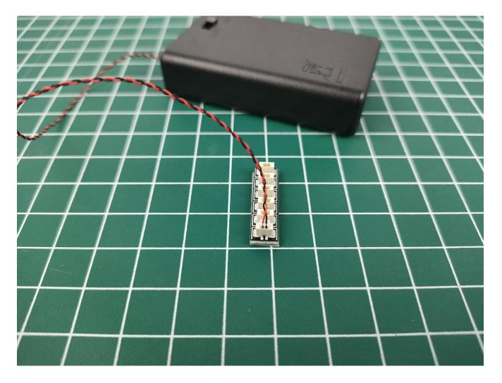
Open the battery box cover, install the battery, pay attention to the positive and negative poles.
