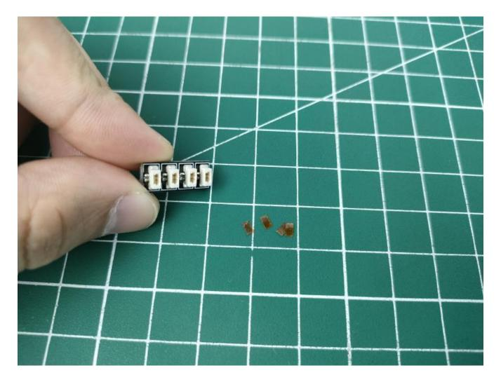
Please pay attention to the use of the interface. The interface is small. Please use it carefully: the = number of the 2P interface is aligned with the = number of the expansion board. The equal sign on the expansion board refers to the two solder joints on the outside, not the two inside the jack Metal pin.
