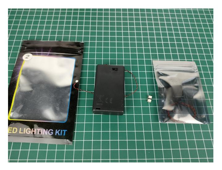
Take out the USB power cord and expansion board from the small bag, the usage is similar to the battery box, you can use the power bank or mobile phone charger head to supply power. The battery box and the USB power cord can be freely chosen, choose one of the two (the USB power cord is used in this article).
